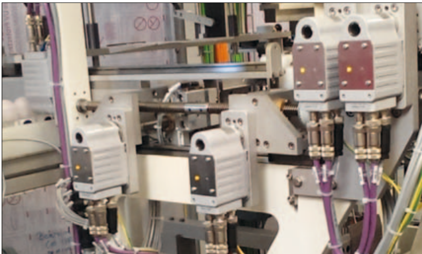
More efficient axis adjustment: The strength of DriveLine is its serial connection – centrally controlled, the SIKO actuators carry out their adjustment assignments synchronously.
