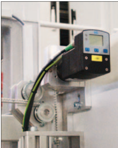
DriveLine actuators ensure precise product position when on-the-fly production change is required.
